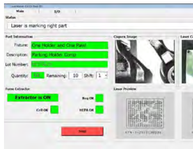
Screen can hide buttons when they shouldn't be used, such as hiding "Start" while marking is in progress.
